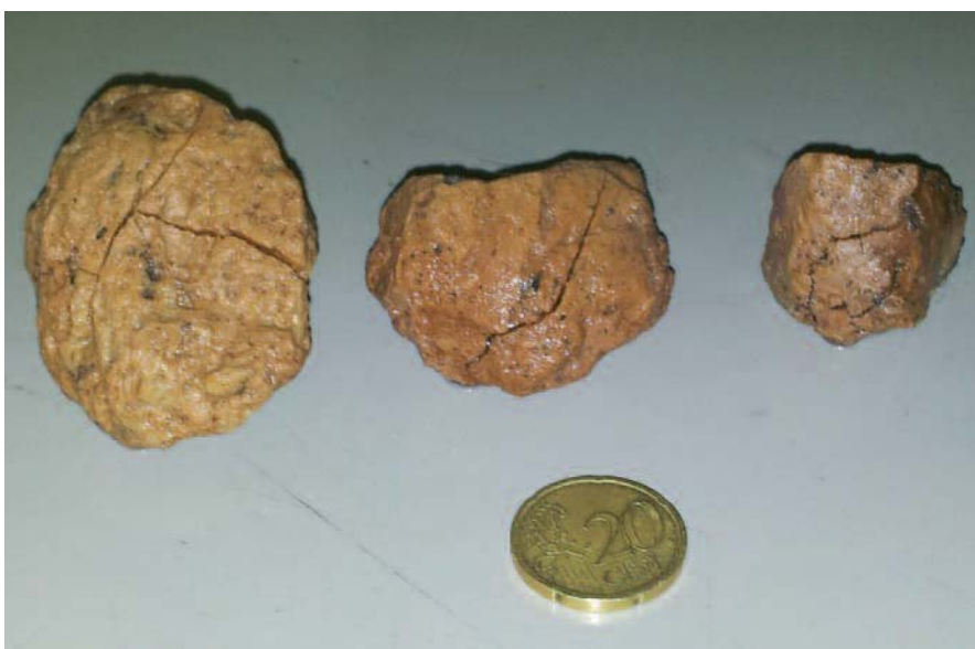
Fig. 2.- Photo shows the fractures displayed in some of the pumice samples. Note: coin is 20 euro cent; 2.20 cm diameter.
