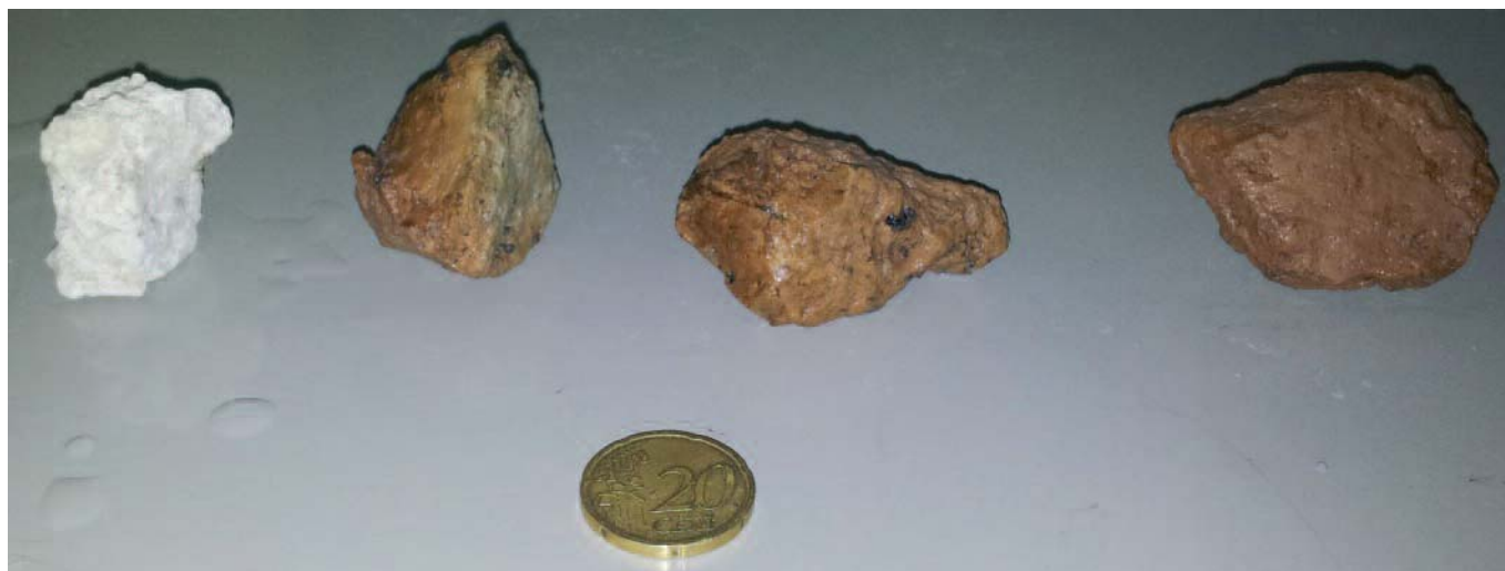
Fig. 1.- From left to right, grading in pumice oxidation from an unaltered sample (with the natural colours) to an extracted at 750°C sample. Note: coin is 20 euro cent; 2.20 cm diameter.
