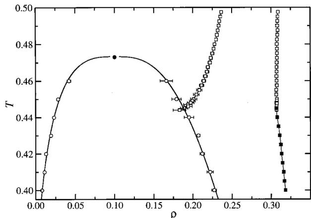
FIG. 8. Fluid–solid coexistence densities for the GB model at low temperatures as obtained from GD integration on lowering the temperature from  $T = 0.50$  (open squares). The filled squares represent solid densities obtained with zero-pressure  $NPT$  simulations. Open circles correspond to the vapor–liquid densities taken from Ref. 11 and the filled circle is the corresponding critical point. The  $V$ – $I$ – $S$  triple point is located at  $T_{VIS} = 0.445$ .
