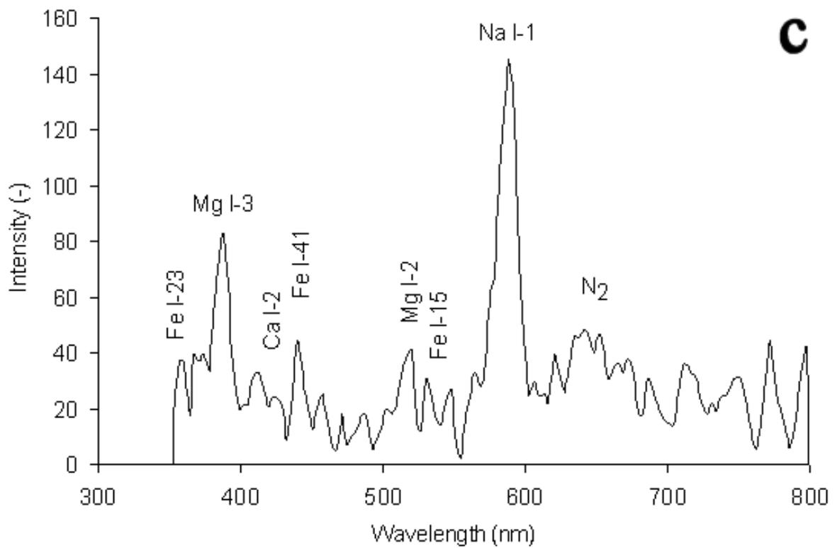
Figure 4. a) Raw and b) calibrated emission spectrum of the Lebrija fireball at time  $t=t_0+0.12$  s ( $t_0$  is the instant of meteor apparition). c) Main lines identified in the spectrum, together with their multiplet number (intensity is expressed in arbitrary units).
