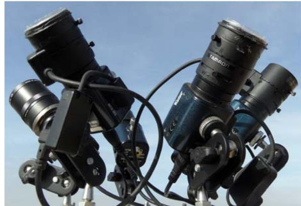
Figure 1. One of the new 6-videospectrographs arrays employed at the Cerro Negro mobile station.
