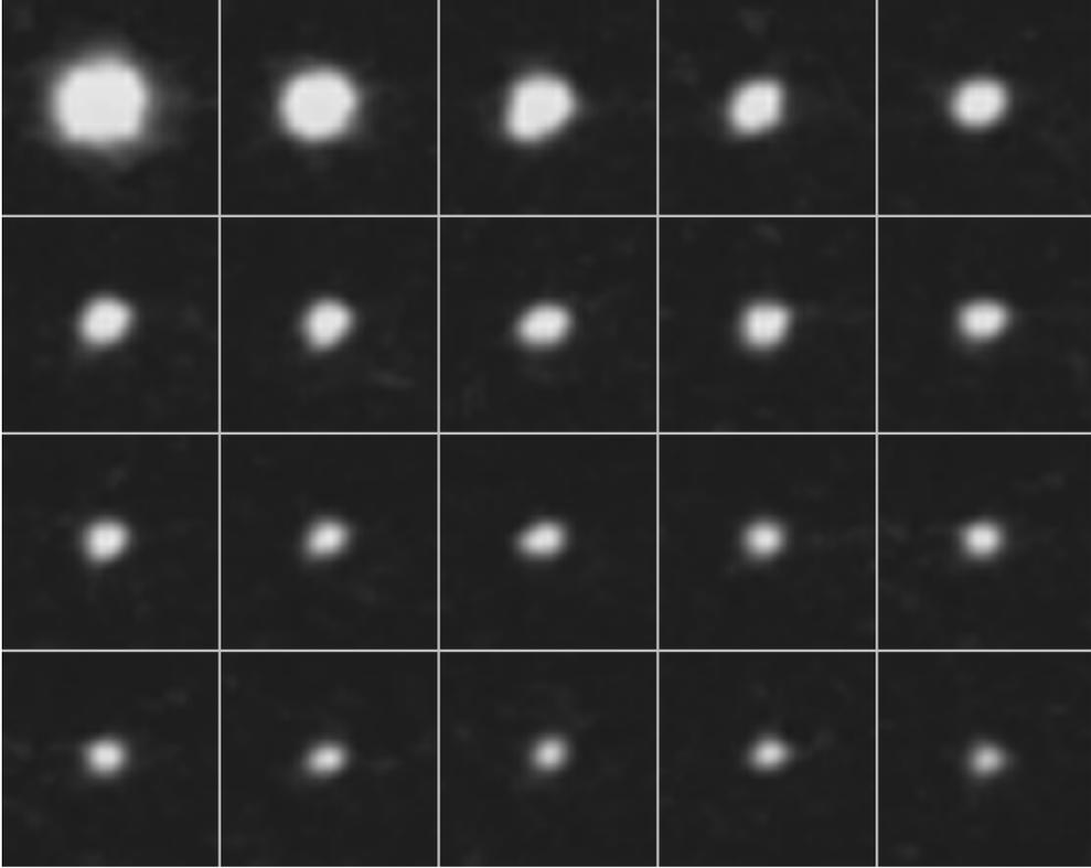
Figure 5. Mosaic of zoomed images showing the flash evolution with time during the first two seconds. Time increases from left to right on each row, starting from the upper left. The time interval between two consecutive images on the same row is 0.1 seconds
