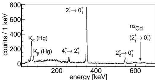
FIG. 2. Random-subtracted  $\gamma$ -ray spectrum of  $^{182}\text{Hg}$  Coulomb excited by a  $^{112}\text{Cd}$  target, Doppler-corrected for the projectile. Intense K X-ray peaks are clearly visible in the spectrum.
