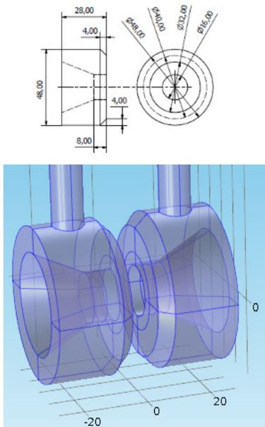
Figure 1: Layout of the buncher consisting of two electrodes fixed by vertical stems.
