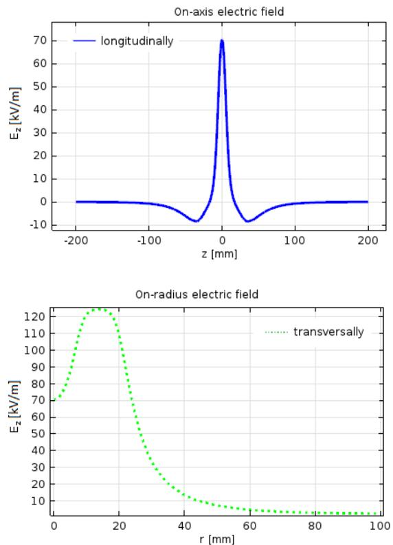
Figure 5: Longitudinal electric field along the beam axis (top) and along the normal to it at  $z = 0$  (bottom).
